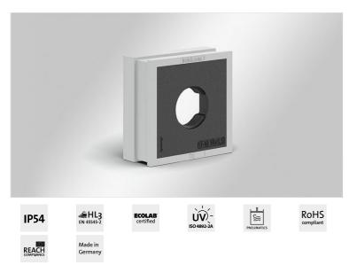
QT-AT-M is an adapter grommet (based on large QT grommets) with integrated metric threads.. The QT-AT-M adapter grommets are made of elastomer with a polyamide body. QT-AT-M adapter grommets are available with inner threads M12 x 1.0, M16 x 1.5, M20 x 1.5 and M25 x 1.5.
